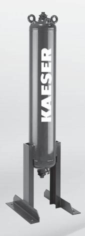
Kaeser's Activated carbon Towers (KAT) are single tower pressure vessels filled with activated carbon adsorbent, that virtually eliminate oil vapor in compressed air. Other hydrocarbon vapors normally adsorbable by activated carbon are also removed.
