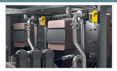
The integrated system comprised of the heat exchanger, thermostatic valve, and complete pipework requires no additional space around the compressor and can recover up to 72% of the overall power consumption of HSD compressors by utilizing the heat in the oil.
