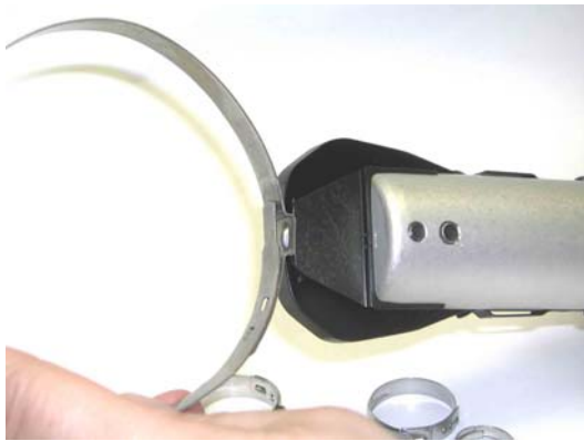
Seen above is a tool developed to close Oetiker™ clamps.
