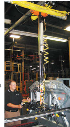
Torque tube with integrated vacuum handling device
