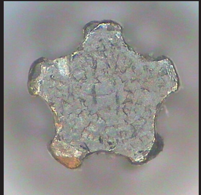
Standard drive bit production: underfilled and severe edge rounding minimises fit and performance.
