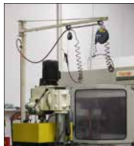
6' Boom Length Application - Shown with optional Hubbell Balancers (see page 8) over machining work area.
