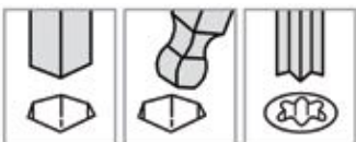
Hex, Ball and Torx® make up the most complete line of key configurations available
