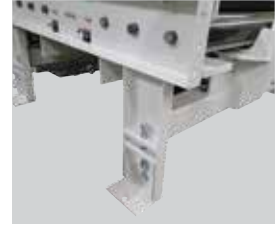
WELDED STRUCTURAL STEEL WITH JACKBOLTS
