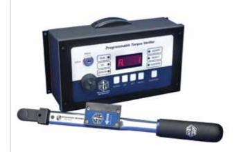
If you are using multiple clicker-type torque wrenches in an assembly cell or need RF communication on job status, the PTV-FM 2.4 GHz offers multiple tool and batch options.
