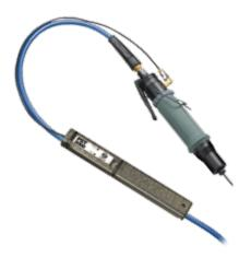
The PST 2000 works with ported auto-shutoff tools to create a profile of the air pressure over time during rundown and shutoff. The profile for a known conforming rundown and tightening is stored on the PST 2000, and all subsequent uses are compared to the profile. Conforming tightenings result in immediate feedback to the operator via an LED display, transmission to the Global Process Monitor, and confirmation on the display and LED's on the Process Monitor unit.
