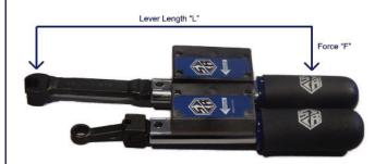
Here is an example of two click wrenches, set to identical settings. If they had the same head length the output would be the same. But, one wrench has an extended head length and that increases the over all lever length. That change in lever length changes the output of the wrench.
