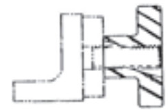
Straighten knob to engage threads for clamping.
