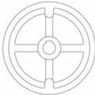
Bored Hole with Keyway
