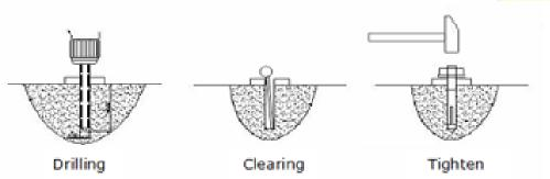
**Anchor Bolt:** <sup>3</sup>/<sub>4</sub>" x 10" Long [Each bolt will provide 150 ft lbs of torque]
