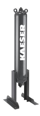
KAESER's Activated carbon Towers (KAT) are single tower pressure vessels filled with activated carbon adsorbent, that virtually eliminate oil vapor in compressed air. Other hydrocarbon vapors normally adsorbable by activated carbon are also removed.
